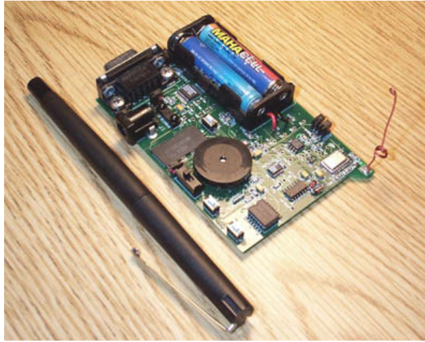
Fig. 1. A SpotON Ad-Hoc Location Sensing Tag
