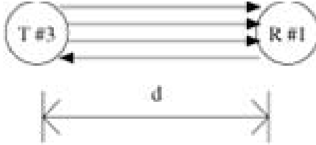
Fig. 10. Receiver #1 is calibrating transmitter #3 at distance d .
