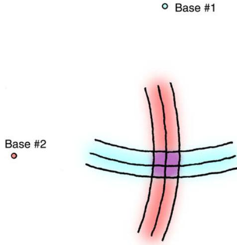
Figure 1: In this hypothetical 2D distance-measurement location system, low dilution of precision occurs because the measurement points have good separation from each other relative to the object being located – conceptually, the area of uncertainty in the intersection is small.
