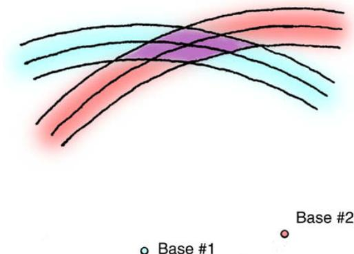
Figure 2: In this hypothetical 2D distance-measurement location system, high dilution of precision occurs because the measurement points have poor separation from each other relative to the object being ranged. The *distance* measurement error is the same as in Figure 1, but the location uncertainty will be larger.
