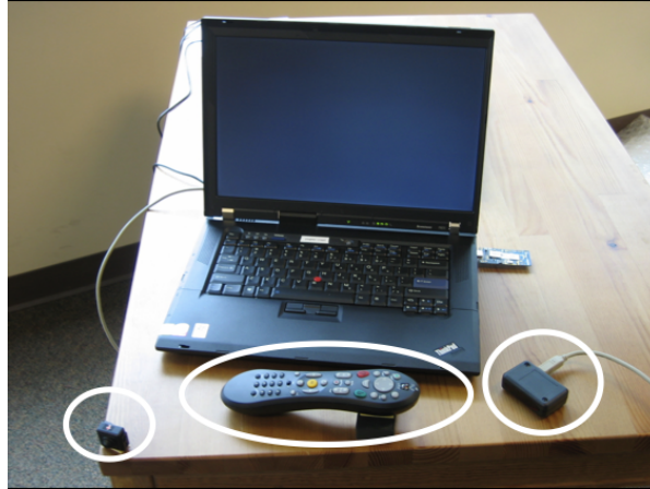
Fig. 1: Data Collection Components: top, laptop receives sensor streams, trains and runs the classifier, and graphically displays the results; bottom left to right, video camera captures a live view of the room from the television’s perspective, remote control with attached accelerometer module attached, universal infrared code receiver.
